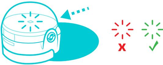
Ozobot will move forward and blink green, which means it has successfully calibrated. Start over if Ozobot blinks red.
